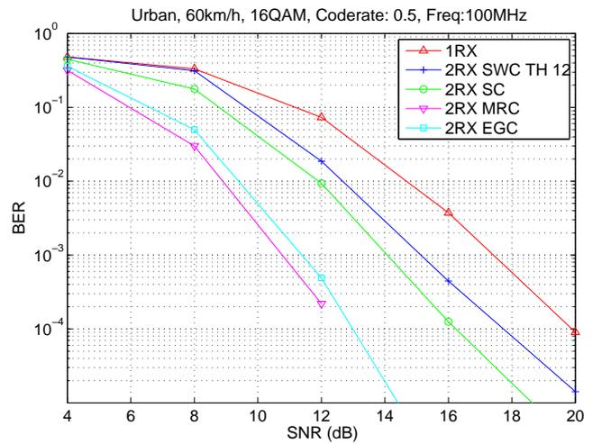
Figure 2: Simulation results for an urban channel
