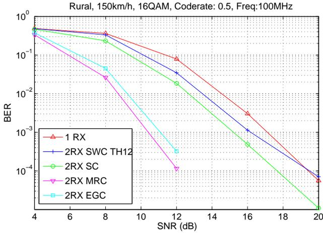
Figure 3: Simulation results for a rural channel
