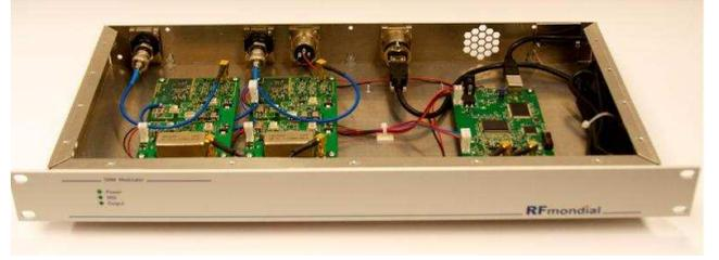
Figure 4: Diversity DRM+ receiver prototype
