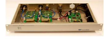
Figure 4: Diversity DRM+ receiver prototype
