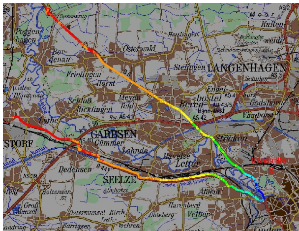
Figure 2: Field strength along two of the radials (higher values on blue and lower values on red).
