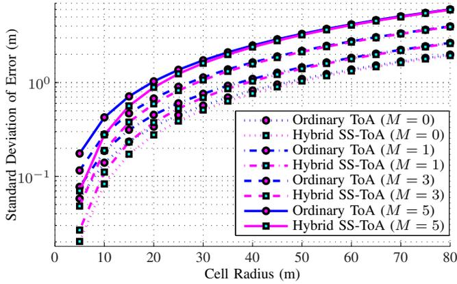
Fig. 5. Cramér-Rao lower bound as a function of cell radius for several numbers of NLoS base stations with  $\text{SNR}_{\text{dB}}$  (signal-to-noise ratio) = 100 dB,  $B$  (number of BSs) = 7,  $\gamma = 2.55$  and  $d_0$  (close-in distance) = 4 m.
