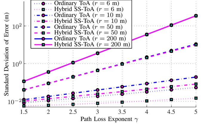
Fig. 3. Cramér-Rao lower bound as a function of the path loss exponent for several cell radii with  $\text{SNR}_{\text{dB}} = 120$  dB,  $\bar{\beta}$  (effective bandwidth) =  $\frac{1}{\sqrt{3}}$  5 MHz,  $B$  (number of BSs) = 7,  $M$  (number of BSs receiving NLoS signals) = 3 and  $d_0$  (close-in distance) = 4 m.
