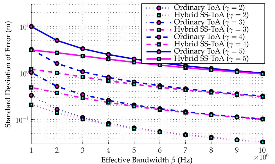
Fig. 2: Cramér-Rao lower bound as a function of the effective bandwidth for several path loss exponents with  $\text{SNR}_{\text{dB}} = 110$  dB, the number of the BSs  $B = 7$ , the number of the BSs receiving NLoS signals  $M = 3$ , the close-in distance  $d_0 = 4$  m and the cell radius  $r = 20$  m.
