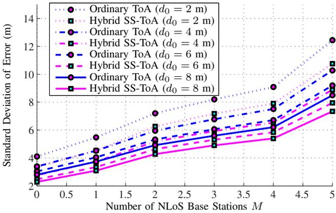
Fig. 6. Cramér-Rao lower bound as a function of the number of NLoS base stations for several close-in distances with  $\bar{\beta}$  (effective bandwidth) =  $\frac{1}{\sqrt{3}}$  5 MHz,  $B$  (number of BSs) = 7,  $\text{SNR}_{\text{dB}}$  (signal-to-noise ratio) = 80 dB, and  $r$  (cell radius) = 20 m.
