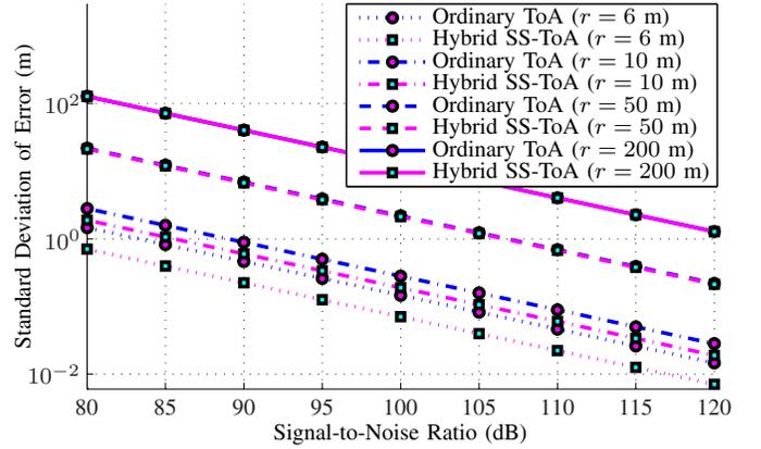
Fig. 4. Cramér-Rao lower bound as a function of the signal-to-noise ratio for several cell radii with  $\bar{\beta}$  (effective bandwidth) =  $\frac{1}{\sqrt{3}}$  5 GHz,  $B$  (number of BSs) = 7,  $M$  (number of BSs receiving NLoS signals) = 3,  $\gamma$  (path loss exponent) = 2.55 and  $d_0$  (close-in distance) = 4 m.
