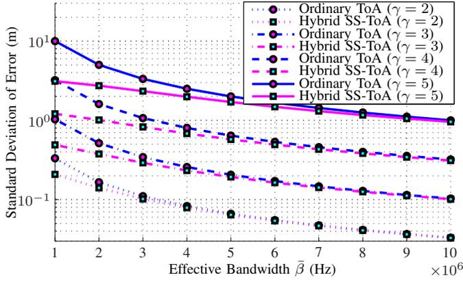
Fig. 2. Cramér-Rao lower bound as a function of the effective bandwidth for several path loss exponents with  $\text{SNR}_{\text{dB}} = 110$  dB,  $B$  (number of BSs) = 7,  $M$  (number of BSs receiving NLoS signals) = 3,  $d_0$  (close-in distance) = 4 m and  $r$  (cell radius) = 20 m.
