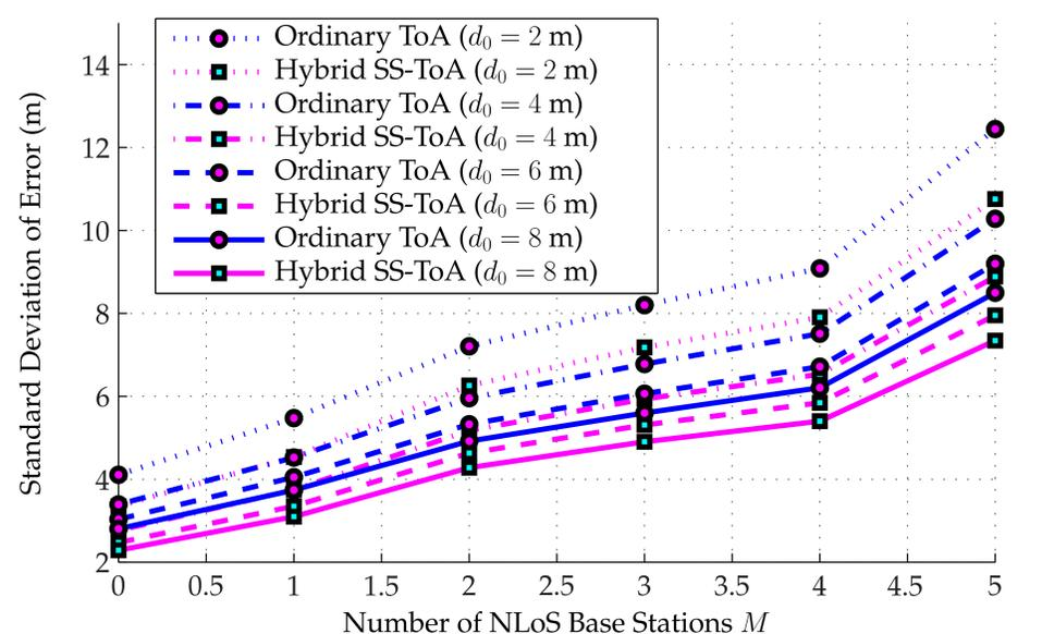
Fig. 4: Cramér-Rao lower bound as a function of the number of the NLoS base stations for several close-in distances with the effective bandwidth  $\beta = \frac{1}{\sqrt{3}} 5$  MHz, the number of the BSs  $B = 7$ , the signal-to-noise ratio  $\text{SNR}_{\text{dB}} = 80$  dB, and the cell radius  $r = 20$  m.
