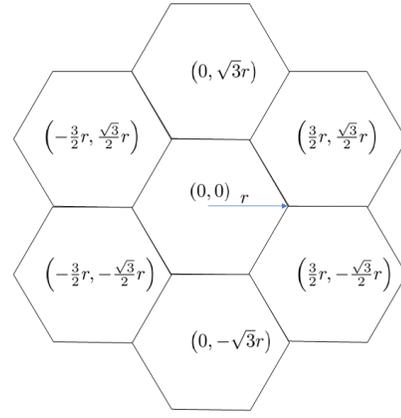
Fig. 1. Cellular system with cell radius  $r$ .
