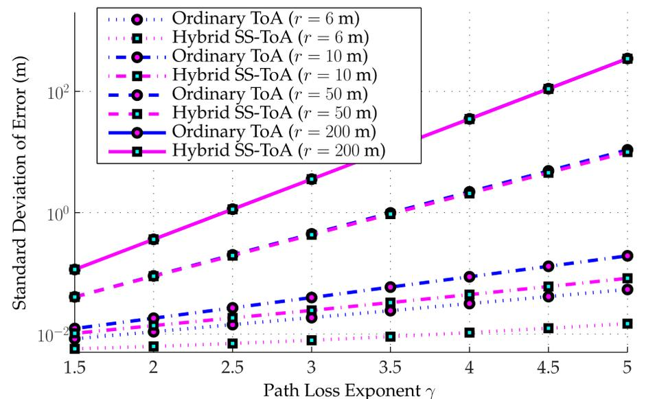
Fig. 3: Cramér-Rao lower bound as a function of the path loss exponent for several cell radii with  $\text{SNR}_{\text{dB}} = 120$  dB, the effective bandwidth  $\beta = \frac{1}{\sqrt{3}} 5$  MHz, the number of the BSs  $B = 7$ , the number of the BSs receiving NLoS signals  $M = 3$  and the close-in distance  $d_0 = 4$  m.
