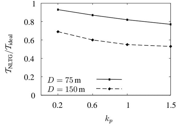
**Fig. 5:** Relative throughput  $T_{\text{NLTG}}/T_{\text{ideal}}$  for  $D = 75 \text{ m}$  and  $D = 150 \text{ m}$
