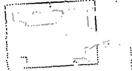
Figure 2: Virtual 2D Scan (black) in comparison to a regular 2D Scan in 20cm height (grey). Scene from (Fig.1)
