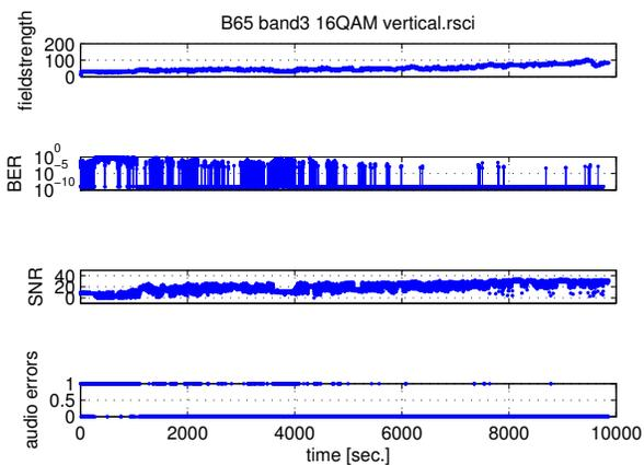
Figure 5. Measurement of the coverage limit in Band III
