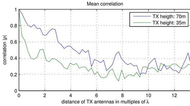
Fig. 3. Mean correlation between the RX signals from 2 vertical polarized TX antennas with different distances
