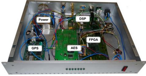
Fig. 6. The hardware setup of the DRM+ diversity transmitter
