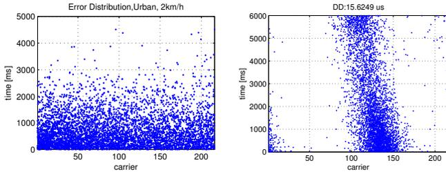
Fig. 1. Distribution of bit errors (blue dots) in an uncoded system in an urban channel simulation with slow receiver velocity (left: without DD, right: with DD)
