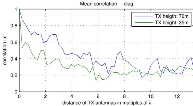
Fig. 4. Mean correlation between the RX signals from 2 diagonal ( $\pm 45^\circ$  slanted) TX antennas with different distances
