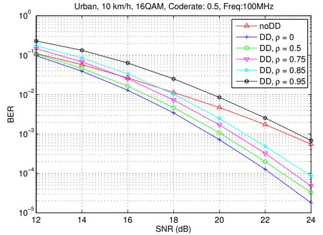
Fig. 2. Simulation of the performance in an 'urban' channel with different correlated paths
