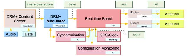
Fig. 5. Block diagram of the transmitters hardware setup
