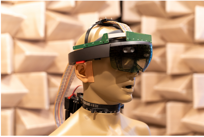
Figure 2: The KEMAR HATS equipped with a Microsoft HoloLens and the 16-channel MEMS microphone array extension.
