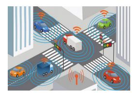
With the development of technology, the awareness area of automatic vehicles has increased in size. Better sensors mean also a wider sensing range of vehicles and also higher comfort and safety for the drivers. Another way to further increase the awareness radius is by using vehicular communication. When vehicles send messages with their current status, these can propagate for hundreds of meters and other traffic participants receiving these messages can get the status of the sender.
